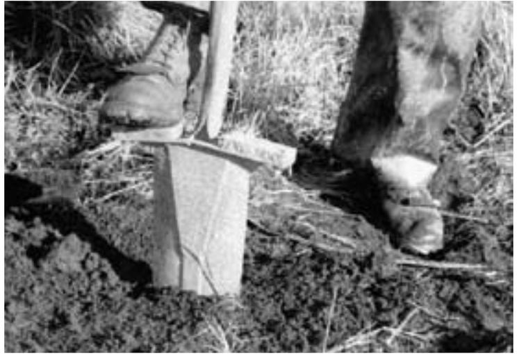
Figure 6.—Shovel sunk one-third into the soil.
